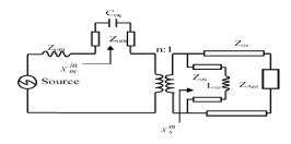
Fig- Equivalent circuit model of vivaldi
