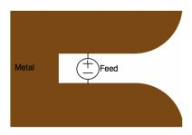
Fig- Geometry of Vivaldi antenna
